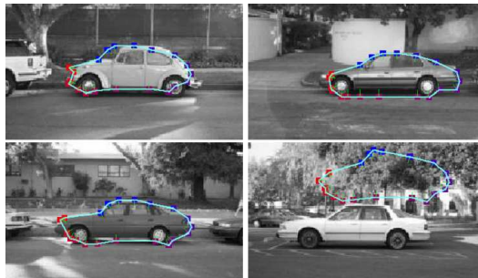
Figure 3: Localization results for the car side object class in the Caltech 101 dataset. Shown are three successful localizations and a single failure. Reasonable localization was achieved in over 85 percent of the test instances.
